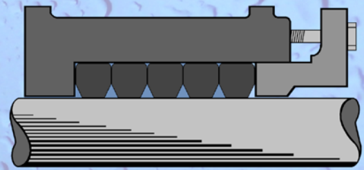
Typical Non-Flushed System
